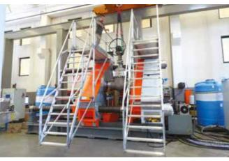
Valve range under testing from 1/2" to 12"
