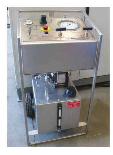
Suitable for hydraulic test up to 4.000 bar or in gas up to 2.500 bar
