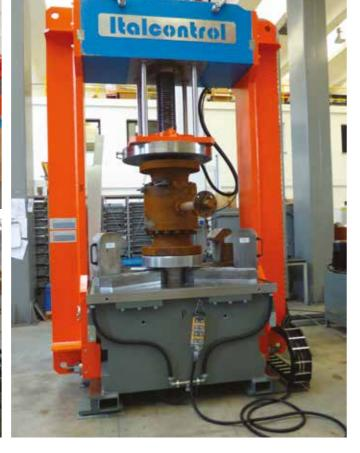
Valve range under pressure testing from 1/2" to 24"
